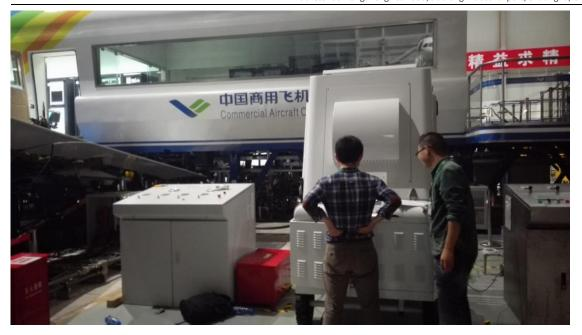
The test bench is designed to test the working characteristics of PMG generator in the flight control system of C919 aircraft. The maximum test speed of the generator is about 24500 r/min, and the system adopts imported high speed and high precision motor to drive directly, which reduces the complexity of the system and greatly improves the maintainability.
